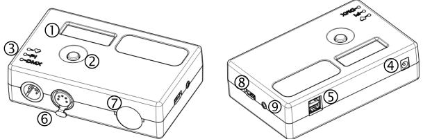
1) <u>LCD DISPLAY</u> This is a text only, 2 lines of 16 characters each, display associated with the *ImageCue*<sup>™</sup> menu system. The display is backlit with a white LED whose intensity can be set through the menu system. During normal operation the display outputs "IMAGECUE" on the top line and "\* \* \* \* \* \* \* \* " on the bottom line. The display also outputs diagnostic messages which are detailed in the Setup section of this guide.
