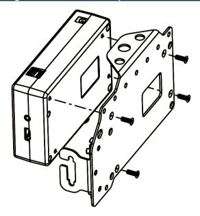
The Mounting Plate and DVI Adapter Bracket assembly kit is supplied with every *ImageCue*<sup>™</sup> unit. The kit includes the mounting plate with the adapter support bracket already attached; an HDMI male to DVI female adapter; and 4 – M4x12 flat head machine screws.
